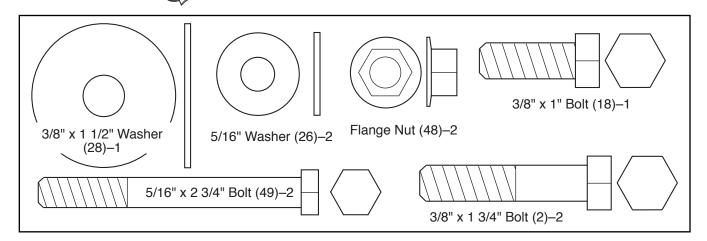
1. Raise the Upright (11) to the vertical position. Insert the 3/8" x 1" Bolt (18), with the 3/8" x 1 1/2" Washer (28), into the lower end of the Upright. Finger tighten the Bolt into the Frame (59).
